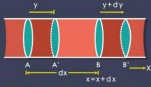
When a longitudinal wave is propagated in a gaseous medium, it produces compression and rarefaction in the medium periodically.
