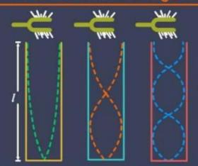
Fundamental frequency of oscillations of closed organ pipe of length I is given as
